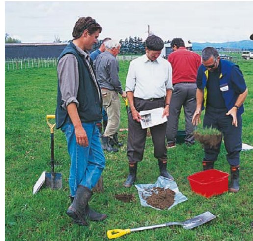
The drop shatter test. The sample is dropped a maximum of three times from a height of 1m (waist height) onto the wooden square in the plastic basin. The soil is then transferred onto the large plastic bag and graded so that the coarsest clods are at one end and the finest aggregates are at the other end.
